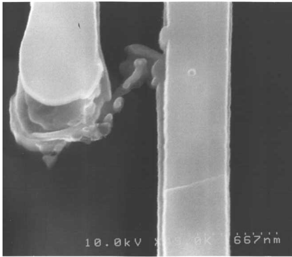
Fig. 5. SEM image of Al wiring short.
